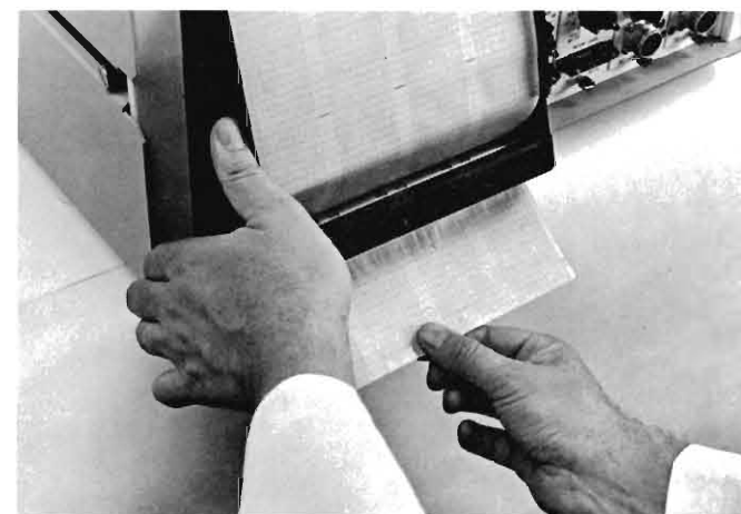
6. CLOSE PAPER TABLE, pulling down slightly on paper. Press table in firmly so it locks in place.
